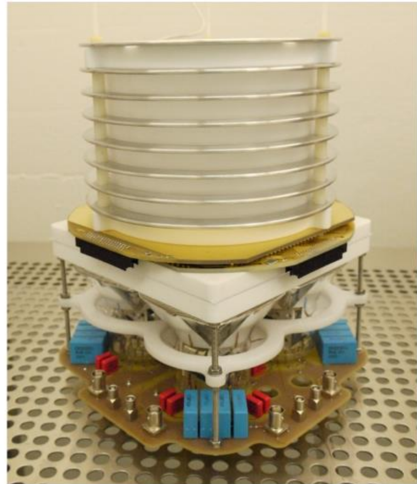
Figure 1: The EXO-100 TPC, shown as a model (left) and assembled. On the left, the parts of the TPC are identified: 1 – detection volume, 1' – cathode, 2 – charge collection system, 3 – light collection system. (Image: S. C. Delaquis [1])
