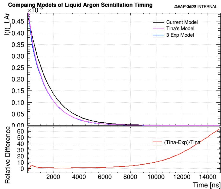
*Fig 10: Comparison between different models for the time structure of liquid argon scintillation with linear axes.*
