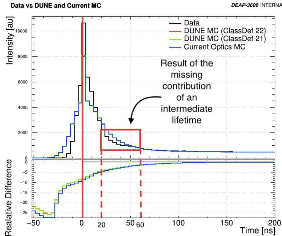
*Fig 5: Pulse shape comparison without intermediate lifetime.*
