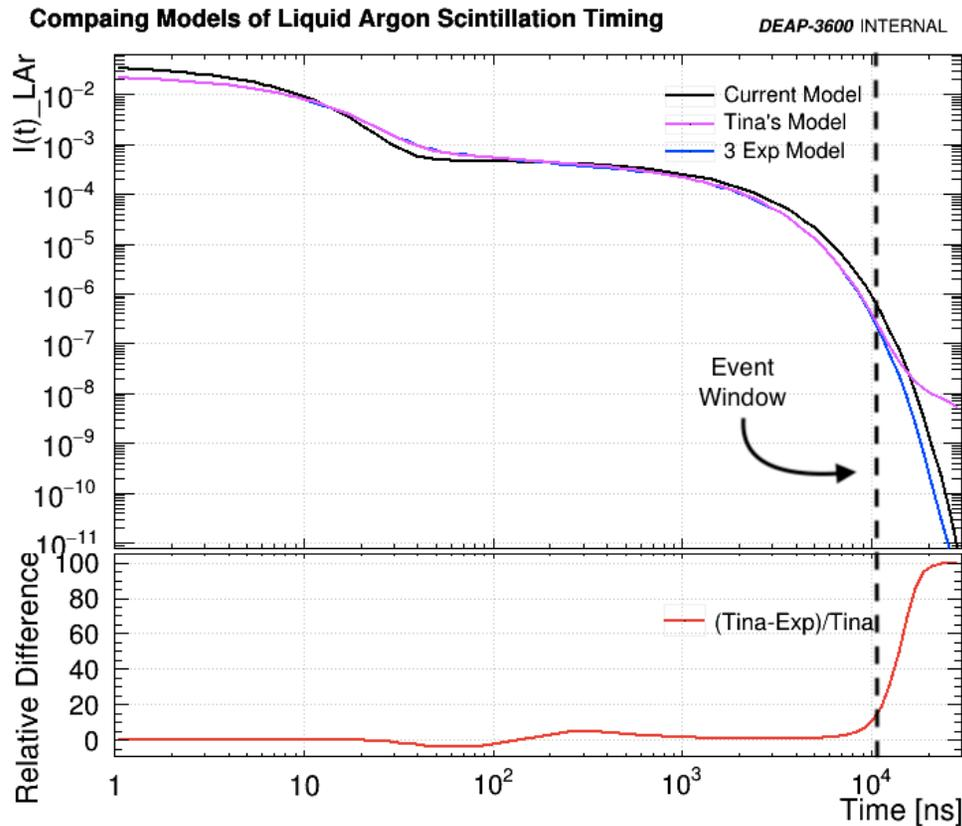
*Fig 7: Comparison between different models for the time structure of liquid argon scintillation.*
