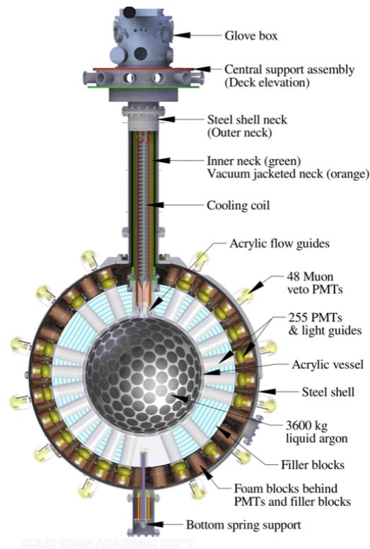
*Fig 1: Cross-section of the DEAP-3600 detector.*
