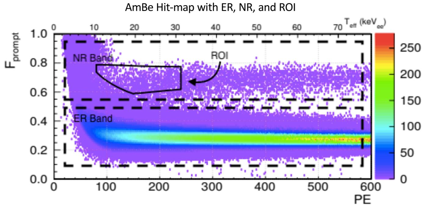
*Fig 2: Hit-map example of ER, NR, and ROI with AmBE source deployed for calibration.*
